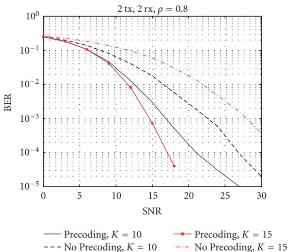
Figure 6.6.  $K = 10$  and  $K = 15$ , ML with/without precoding.
