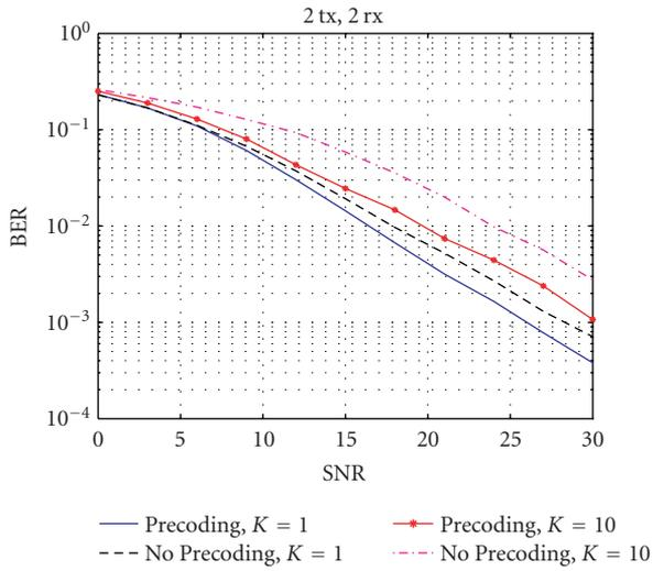
Figure 6.4.  $K = 1$  and  $K = 10$ , MMSE SIC with/without precoding.
