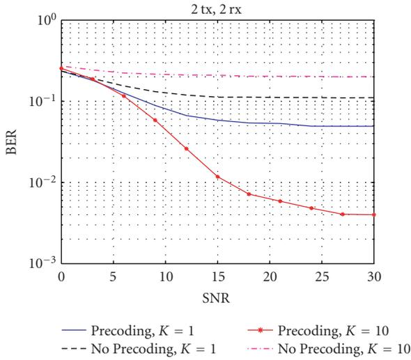
Figure 6.3.  $K = 1, K = 10$ , MRC with/without precoding.
