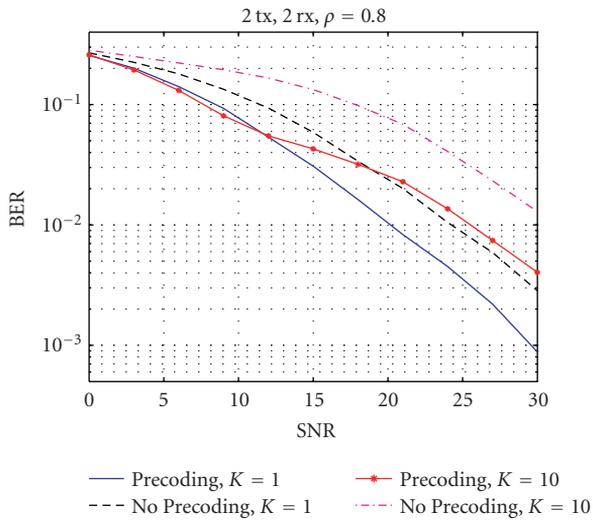
Figure 6.5.  $K = 1$  and  $K = 10$ ,  $\rho = 0.8$ , MMSE SIC with/without precoding.
