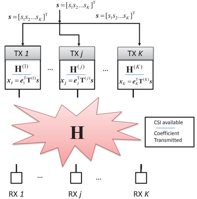
Fig. 1. Distributed precoding in the DCSI-MIMO channel.
