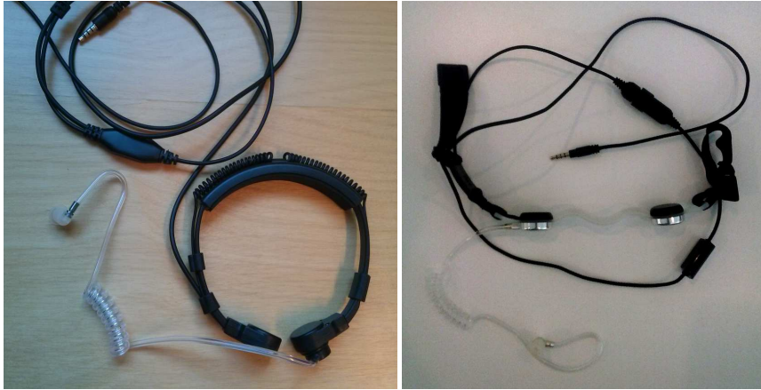
Fig. 7: Throat-microphones used in [141] [Reprinted with permission from IEEEACM Transactions on (T-ASL) Audio, Speech, and Language Processing].
