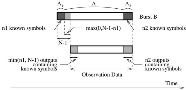
Figure 1: Burst Transmission
