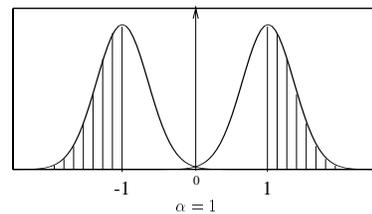
Figure 1: Distribution of the symbol estimates at the output of the MMSE ZF equalizer: reliable decisions such that  $|\hat{a}(k)| \geq 1$
