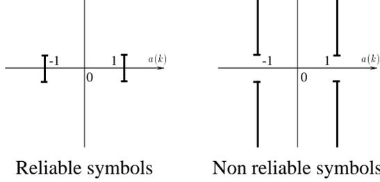
Figure 4: Joint distribution of  $v'(k)$  and  $a(k)$  for the reliable (left) and non reliable decisions (right)
