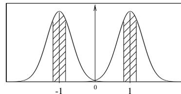
Figure 3: Distribution of the symbol estimates at the output of the MMSE ZF equalizer: reliable decisions such that  $|\hat{a}(k) - \text{dec}(\hat{a}(k))| \geq \beta$
