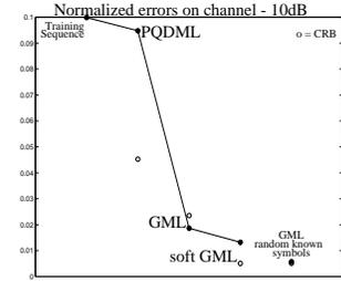
Figure 6: NMSE for semi-blind PQDML, GML and soft GML
