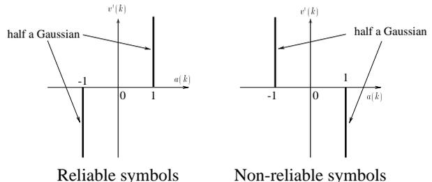
Figure 2: Joint distribution of  $v'(k)$  and  $a(k)$  for the reliable (left) and non reliable symbols (right)
