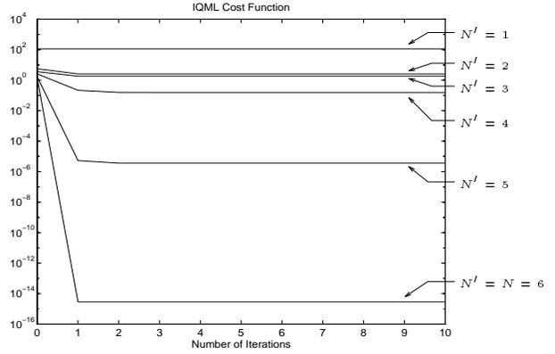
**Figure 6.** Evolution of the averaged IQML cost function during the iterations for  $H1$  and  $N' = 1, \dots, N$ .
