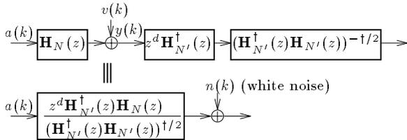
Figure 2. MFB1: reduced-order multichannel MF followed by a scalar MF.
