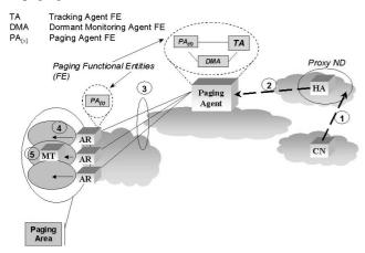
Figure 5: Integration of an IP paging architecture into a Mobile IPv6 managed platform
