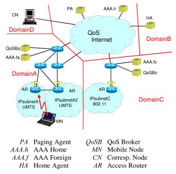
Figure 1: Conceptual view of the heterogeneous network
