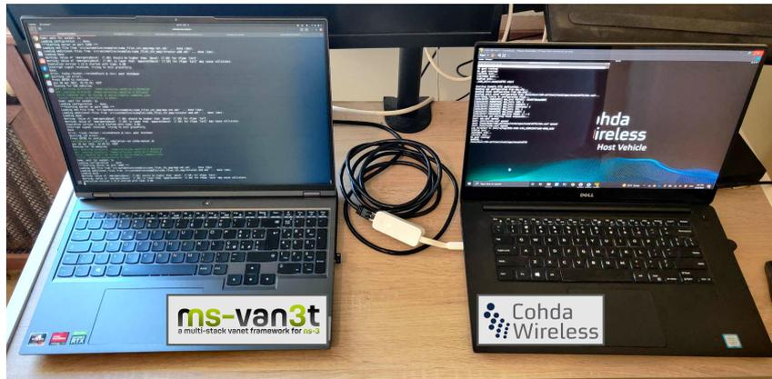
Fig. 3.6 Laboratory setup for the interoperability tests, performed to validate the emulation feature available in ms-van3t.
