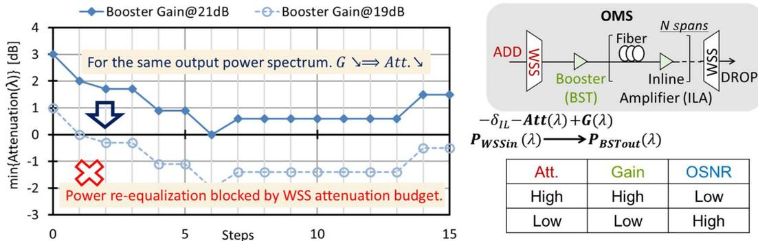
**Figure 1.** WSS attenuation budget blocks power re-equalization. Left: solid dark blue curve is the experimental results [3] with proper gain setting, dash light blue curve represents the fact that there'll be no attenuation budget with a non-proper gain setting.
