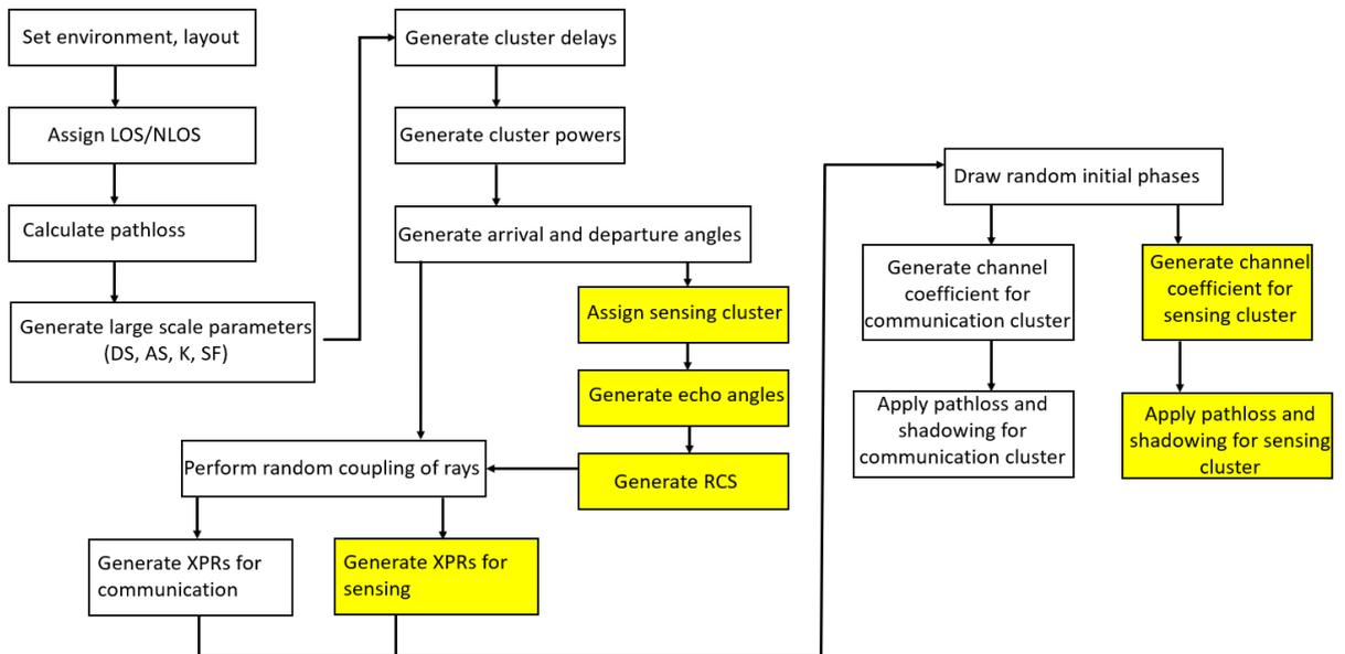
**Figure 1. Channel coefficients generation procedure for communication and sensing channels.**
