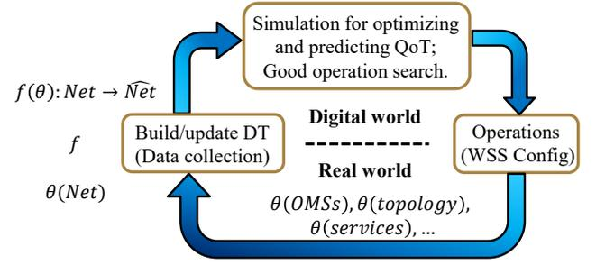
Fig. 4. Digital twin enabled power equalization.
