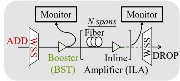
Fig. 2. Optical multiplexing section.
