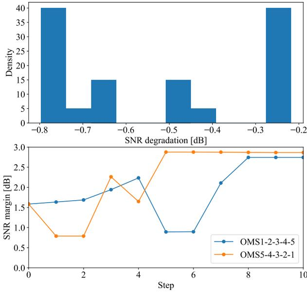
**Fig. 6.** SNR degradation with open-loop. Top: Simulation results of SNR degradation value with 120 different orders. Bottom: SNR margin variation with different operation orders.
