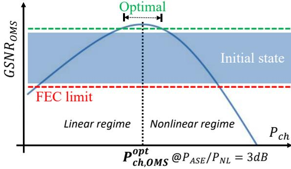
Fig. 3. GSNR and optimal launch power at  $P_{ASE}/P_{NL} = 3dB$ .
