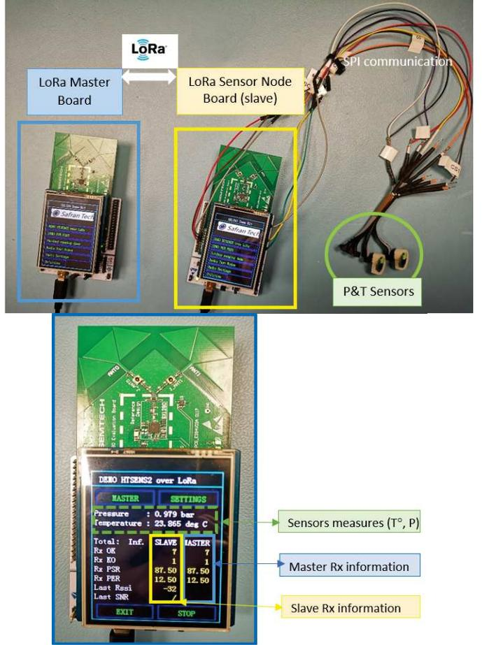
Fig. 2: (a) P&T Wireless Sensing Network based on a LoRa communication, (b) Performances displayed on the LoRa master board
