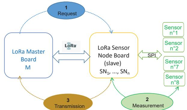
Fig. 1: A wireless sensing network communicating with LoRa modulation between a LoRa master board and a LoRa sensor node board
