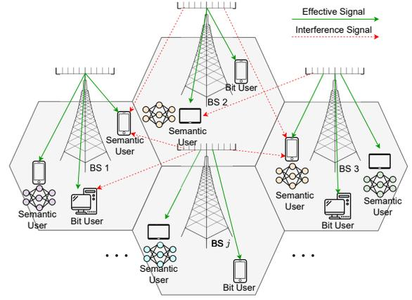
Fig. 1. Example of the proposed semantic-bit coexisting communication for the multi-cell multi-user MIMO system.
