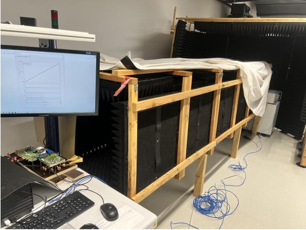
Fig. 2. Radar measurement setup: FMCW radar module, RF transmission tunnel, and RTS.
