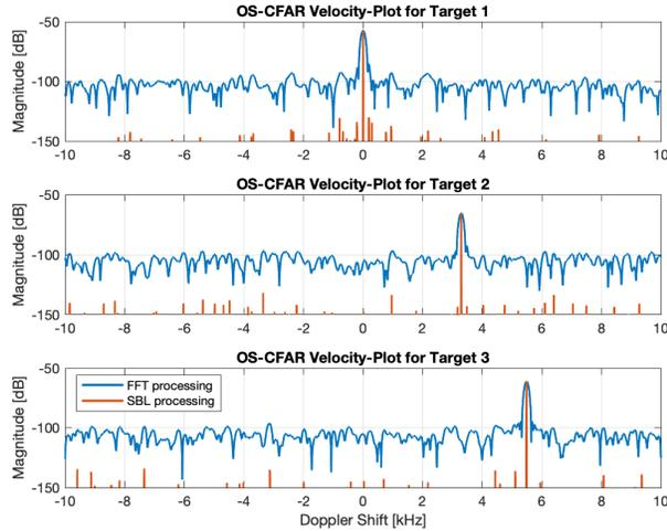
Fig. 5. Doppler shift estimation from experimental data for the same three radar targets as in Fig. 4. FFT-based power spectral density estimate (blue) and SBL-based processing (red).
