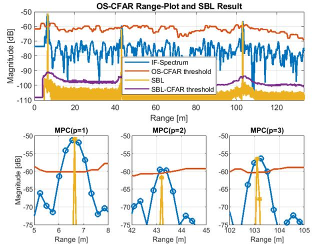
Fig. 4. Range estimates from experimental beat-frequency data for three radar targets. Top FFT-based power spectral density estimate (blue), CFAR-threshold (red), and SBL-based processing (yellow). The bottom plots zoom in on the three radar targets.
