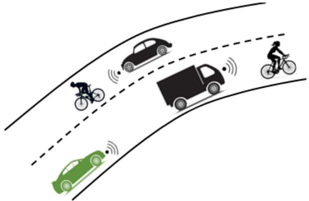
Fig. 1. Traffic scenario with NLOS between the green car and a bicycle.
