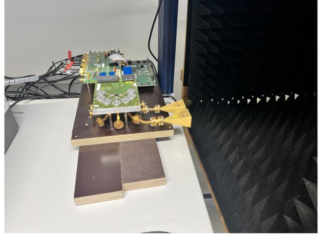
Fig. 3. Radar Measurement setup: FMCW radar module FE.
