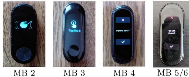
Figure 3.3: Mi Bands pairing confirmation messages. To accept pairing, a user must either press a hardware button (Mi Band 2/3) or touch a software button (Mi Band 4/5/6). Note that Amazfit Cor 1/2 use similar pairing confirmation messages.
