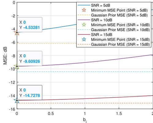
Fig. 4.  $MSE_{x_i}$  with  $x_i = 1$  of Laplacian prior.
