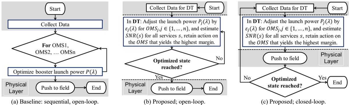
Figure 1. Work flow for the power re-optimization algorithms.
