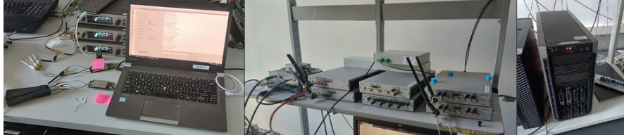
Figure 7: synchronized setup from left with the UE module, multi USRPs connected to the grand master clock by a switch and the gNB machine
