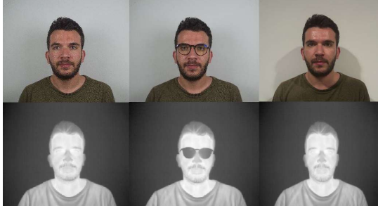
Fig. 2. Example images obtained with Flir Duo R camera. The three variations are displayed in visible (upper row) and thermal (bottom row) spectra, from left to right: N, O and A.
