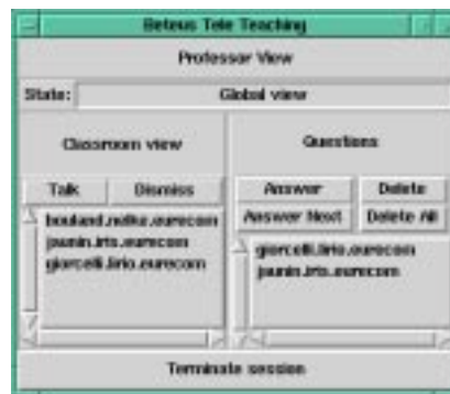
Fig. 8. Directory service window of the control panel user interface.
