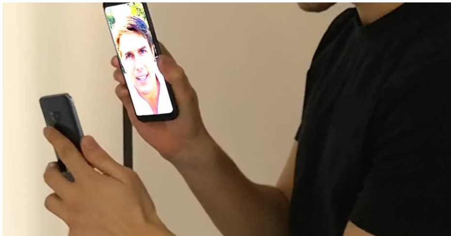
Figure 1: Presentation attack with a screen. One of the smartphones displays a face image to attack a remote KYC application running on the second smartphone.
