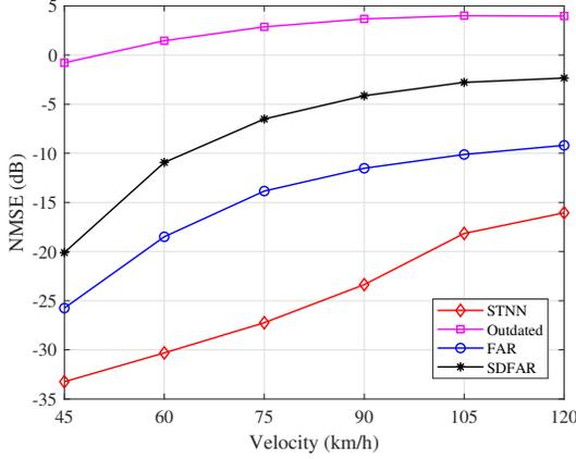
Fig. 8: Comparison of NMSE (dB) between STNN, FAR, SDFAR and linear regression with respect to the velocity  $v$ . The corresponding normalized Doppler shifts  $f_n$  are 0.075, 0.1, 0.125, 0.15, 0.175 and 0.2.
