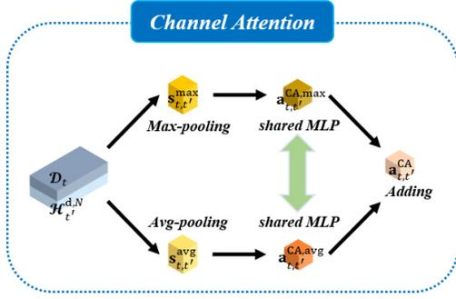
Fig. 4: Diagram for calculating the channel attention weights.
