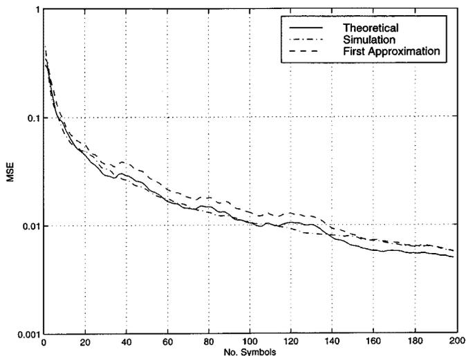
Fig. 2. MSE evolution versus  $N_s$ . Empirical MSE, theoretical MSE given by (58), and a “first approximation” of the MSE obtained via (33), as explained in Section VI.
