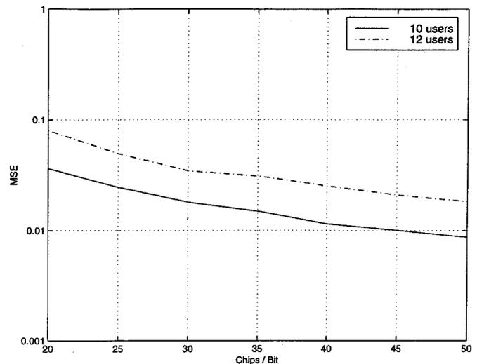
Fig. 3. MSE versus spreading gain.
