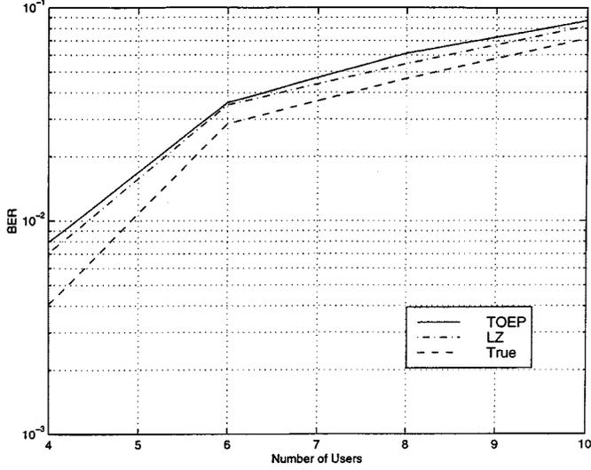
Fig. 7. Bit error rate versus the number of users.
