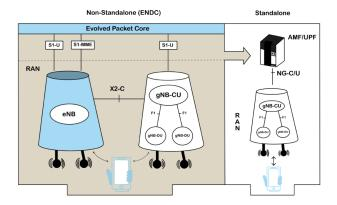
Fig. 3. OAI 5G RAN project showing the architecture for 5G NSA and SA.
