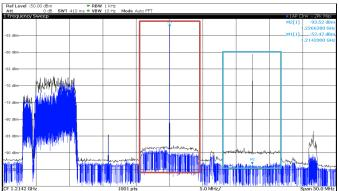
Fig. 12. Transmitting and receiving satellite spectrum from gNB (left; red) and UE (right; blue).
