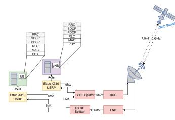
Fig. 6. 5G NTN architecture (*noS1* mode) for the field trial. Our demonstrator includes adapted PHY, MAC, and RLC layer for OAI.
