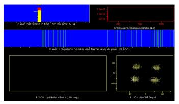
Fig. 9. OAI GUI: QPSK constellation diagram of the PUSCH at the NTN gNB (bottom right).
