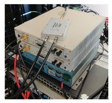
Fig. 8. Two Ettus X310 URSPs functioning as both the gNB and the UE in the NTN demonstration.
