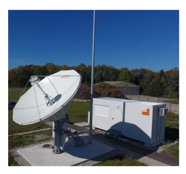
Fig. 7. GEO transmissions with a 4.9 m satellite antenna and co-located gNB and UE in the laboratory building.
