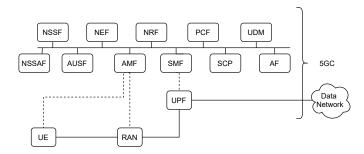
Fig. 4. High level 5G SA architecture.
