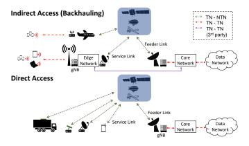
Fig. 2. High level 5G NTN architectures for the indirect access (backhauling) and the direct access. The direct access architecture utilizes the NR waveform on both, feeder link and service link. A direct access UE is sending data over the SatCom link without relay in between.
