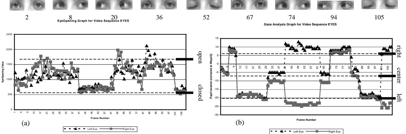
**Figure 1.** Analysis Graphs for a tested sequence. (a) *EyeOpening* (two quantization levels). (b) *GazeDetection* (three quantization levels).
