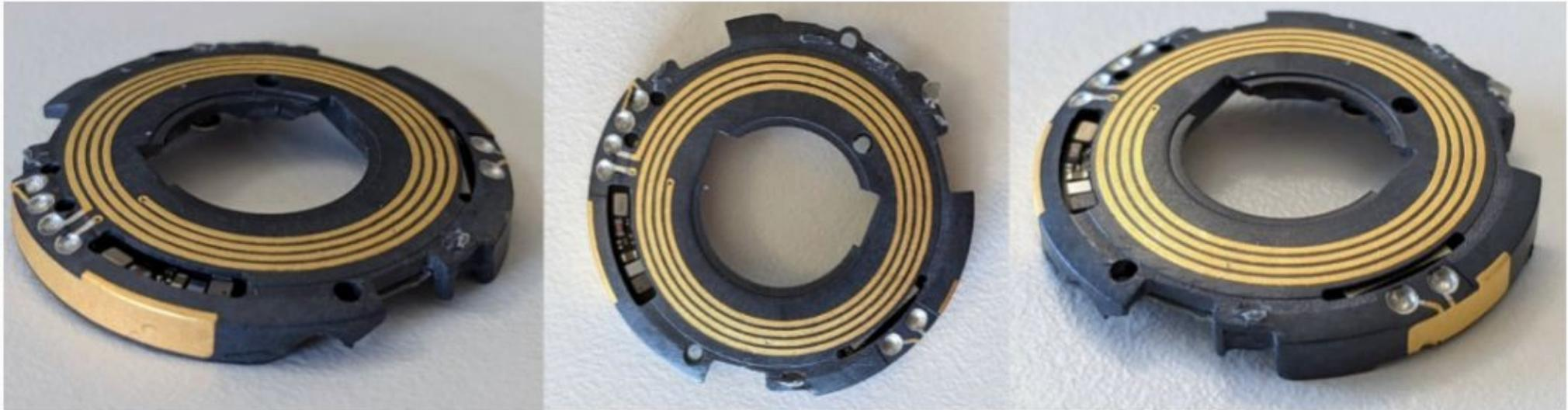
They are all etched onto a single piece of plastic using Laser Direct Structuring (LDS) and then soldered to the PCB around the edge. The NFC antenna also has a short trace on the other side of the plastic (connected with a via at each end) to return the inside end of the coil to the PCB.
