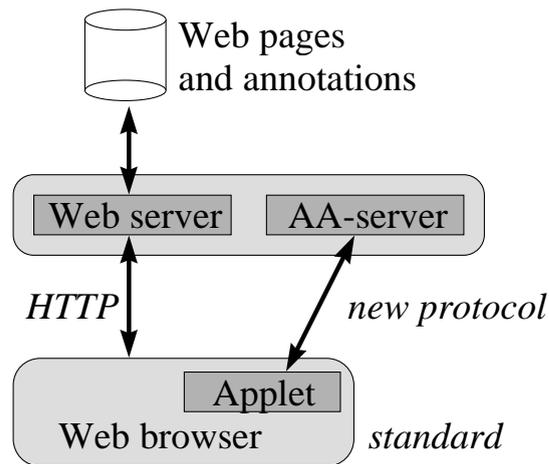
Figure 7 : Architecture of the active annotation service. The Web server is not altered, but accompanied by the active annotation server. The access to the server is handled by an applet thus that the browser does not need to be changed.
