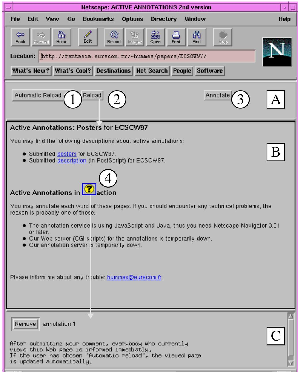
Figure 4 :Screenshot of the active annotation service. The Web page is divided in three frames ; A is the control frame of the annotations service and holds the controls for the selection of the notification strategy (1), a reload button (2), and the annotate button (3). Frame B incorporates the Web page that may be annotated. Annotations are displayed in frame C, when the user presses an annotation link (4) in the Web page.
