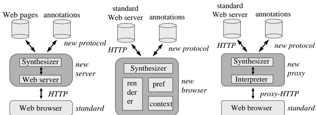
Figure 2 : Three different architectures to merge annotations with the viewed Web pages. The left architecture changes the web server, the middle architecture the browser to synthesize the annotations, which are kept in a separate database with the viewed pages. The proxy of the right architecture places a proxy in the HTTP stream that alters the original stream to combine it with the annotation; the produced output is again conform with the HTTP protocol.
