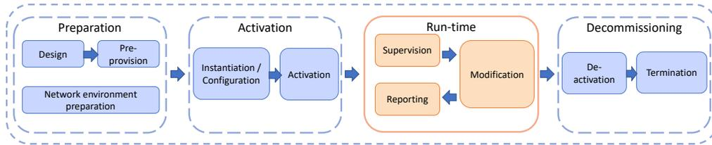
Figure 3: Lifecycle phases of a Network Slice Instance [9]
