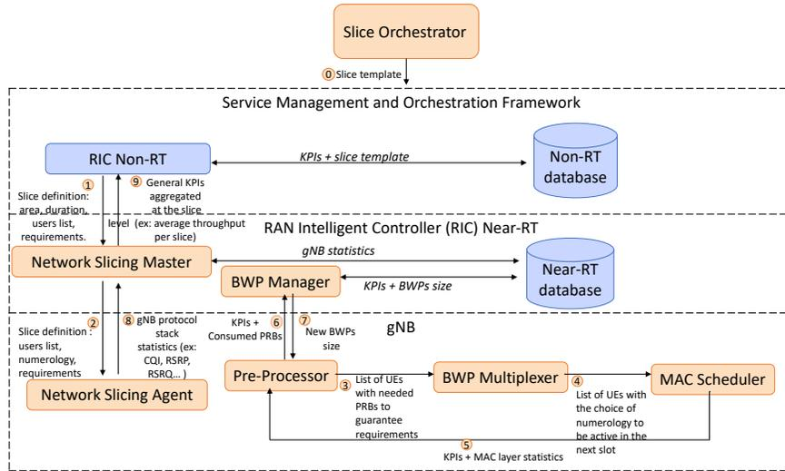
Figure 5: NRflex components mapped to the O-RAN architecture
