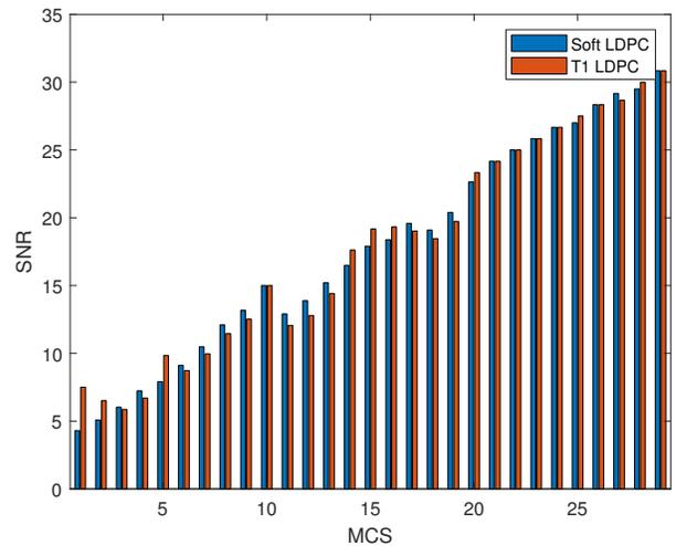
Fig. 7. Soft LDPC and LDPC offload comparison of the SNR required to achieve a 10% BLER in the first round in TDL-C channel with 30ns delay spread.
