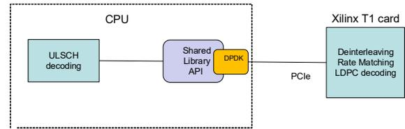
Fig. 4. New architecture using offloading to T1 card.
