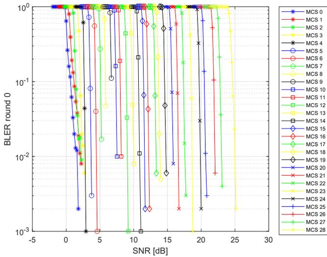
Fig. 5. Soft LDPC decoder block error rate (BLER) of the first round for all MCS in AWGN channel.
