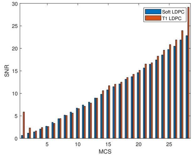
Fig. 6. Soft LDPC and LDPC offload comparison of the SNR required to achieve a 10% BLER in the first round in AWGN channel.
