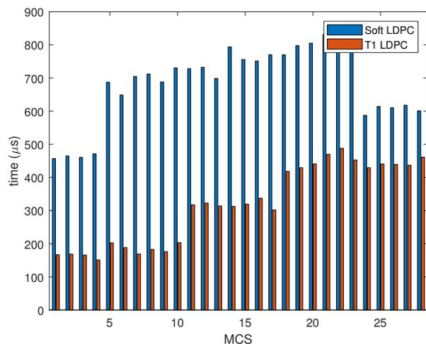
Fig. 8. Soft LDPC and LDPC offload comparison of the average decoding time for each MCS in AWGN channel.
