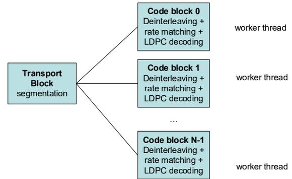
Fig. 3. Current parallel architecture of LDPC decoding.
