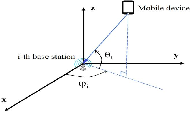
Fig. 1: Uplink DoA at the  $i$ -th base station in the  $xyz$  coordinate system
