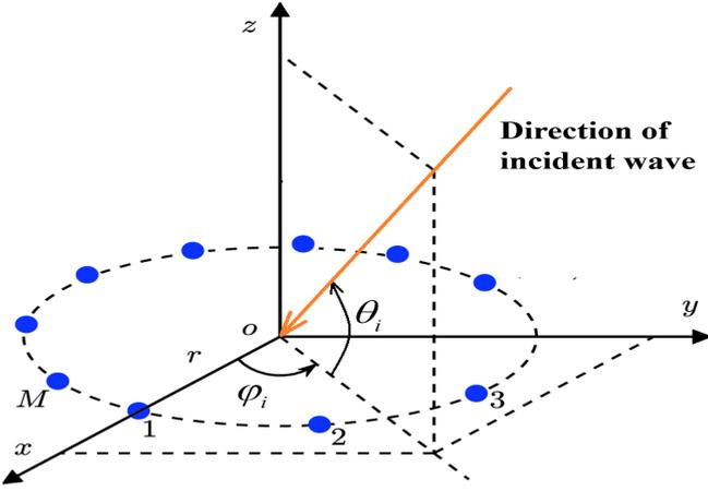
Fig. 4:  $M$ -element Uniform Circular Array (UCA) with radius  $r$  at the  $i$ -th base station to estimate azimuth angle  $\varphi_i$  and elevation angle  $\theta_i$
