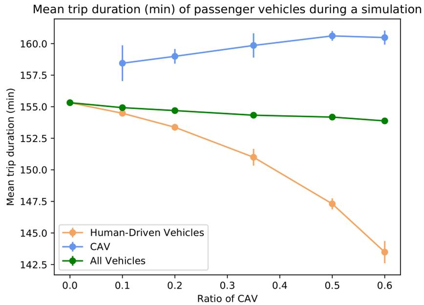
Figure 5: Mean trip duration of vehicles during a simulation
