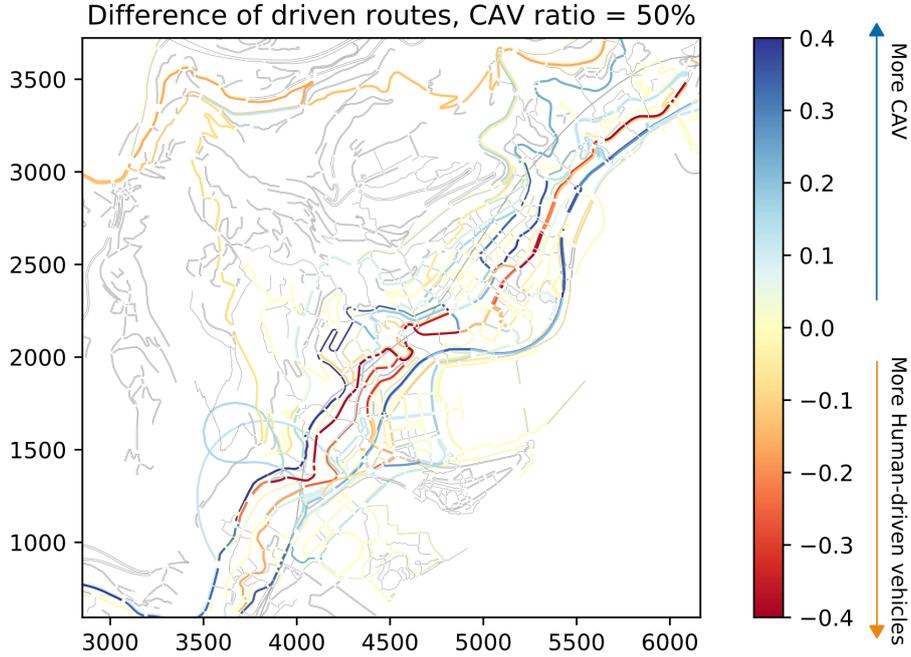
Figure 3: Difference of routes between CAV and human-driven Vehicles for a ratio of CAV of 50%
