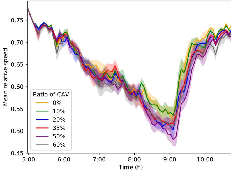
Figure 8: Evolution of the mean relative speed of vehicles through a simulation
