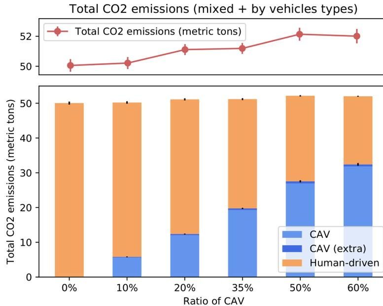
Figure 10: Total CO<sub>2</sub> emissions by vehicle type in a simulation
