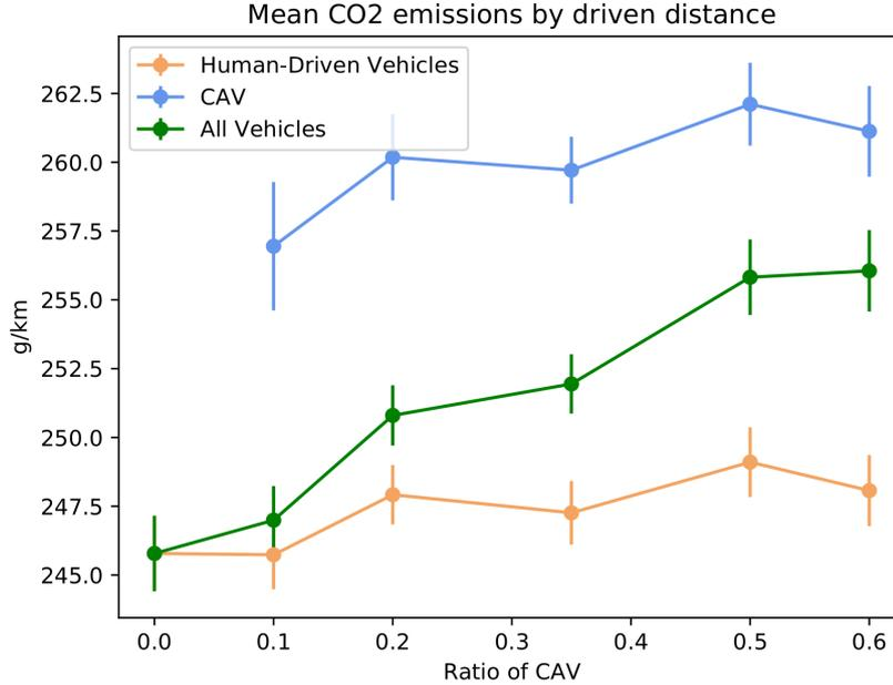
Figure 9: Evolution of the emissions of CO<sub>2</sub> by driven distance by vehicle type
