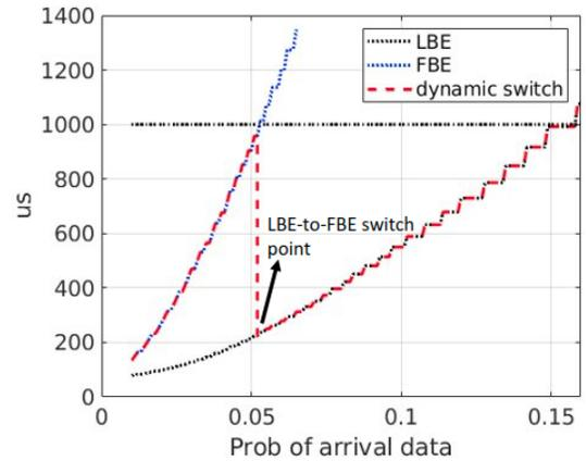
Fig. 4. Channel access time of a UE using FBE, LBE and dynamic-LBE-to-FBE-switch scheme.
