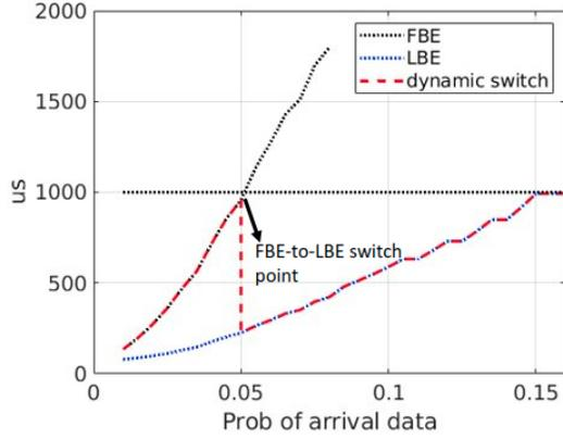
Fig. 2. Channel access time of a UE using FBE, LBE and dynamic-FBE-to-LBE-switch scheme.
