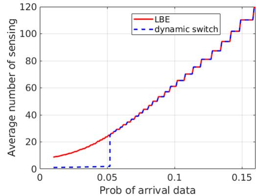
Fig. 5. Number of channel sensing of a UE using LBE and dynamic-LBE-to-FBE-switch scheme.
