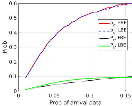
Fig. 3. Probability of sensing a busy channel and transmission probability of a UE using FBE and LBE.
