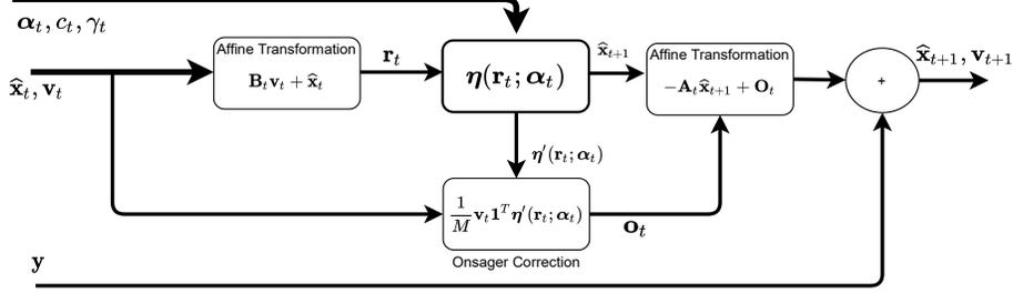
Fig. 1. Block diagram representing one iteration of LAMP-SBL.
