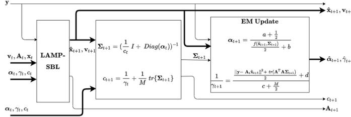
Fig. 2. A single layer of EM-LAMP-SBL. Thicker lines in the diagram represent multiple variables.
