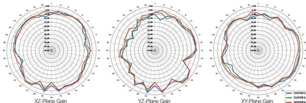
Fig. 3. Antennas gain plots on 3.5GHz
