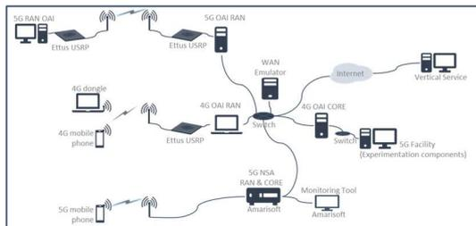
Fig. 1. The 5GENESIS Portable Demonstrator.
