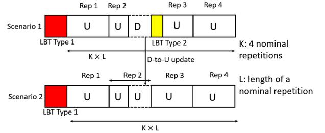
Fig. 4. Semi-static DL symbols are switched to UL symbols.
