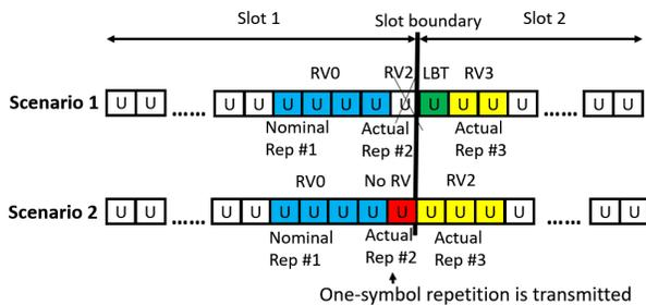
Fig. 5. Orphan-symbol actual repetition containing DMRS is transmitted in unlicensed spectrum.
