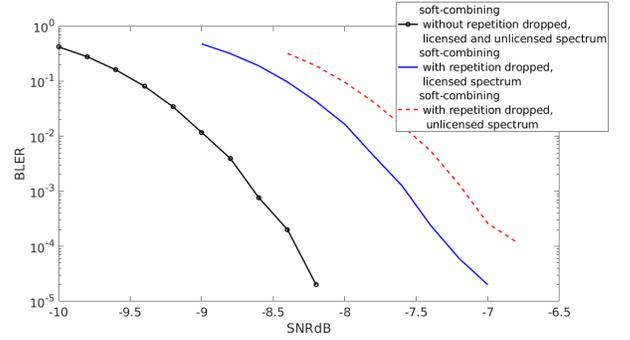
Fig. 8. Performance PUSCH repetitions in licensed and unlicensed spectrum with flexible symbols used as UL symbols
