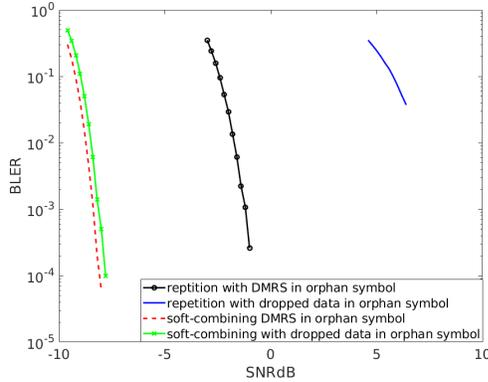
Fig. 9. Performance PUSCH repetitions in unlicensed spectrum with DMRS in orphan symbol
