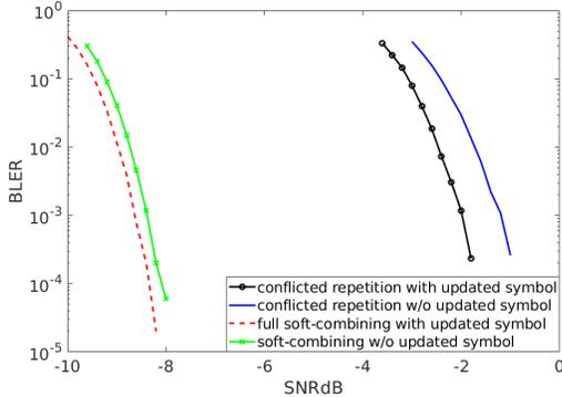
Fig. 6. Performance PUSCH repetitions in licensed spectrum with updated DL-to-UL symbol.
