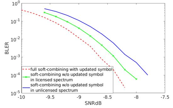
Fig. 7. Performance PUSCH repetitions in unlicensed spectrum with updated DL-to-UL symbol
