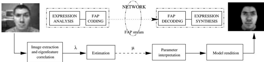
Figure 4: Face animation diagram. The user is recorded by a camera, and an expression analysis system generates the face animation parameters (FAP,  $\mu$ ) which are sent over the network. A decoder interprets them and synthesizes the expressions on the clone.
