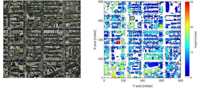
Fig. 4. (Left) An orthoimagery of an 800 [m] \times 800 [m] area in Washington DC, USA. (Right) The corresponding elevation map of buildings and vegetation. The BS is placed at the red triangle with 45 meter height.
