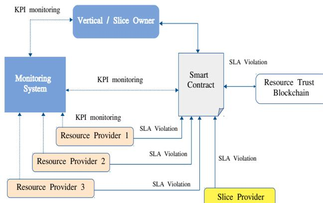
Fig. 1: SLA Management trust architecture
