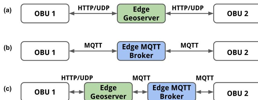
**Figure 7.** The representation of the test cases with two experimental OBUs. Each test case consists of a different combination of V2X communication protocols between both OBUs and the edge cloud.
