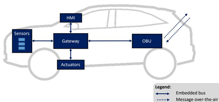
Figure 5. Overview of DS7 vehicle's embedded system.
