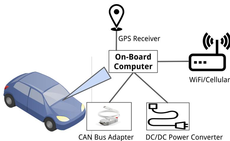
Figure 4. Basic hardware components of the OBU.
