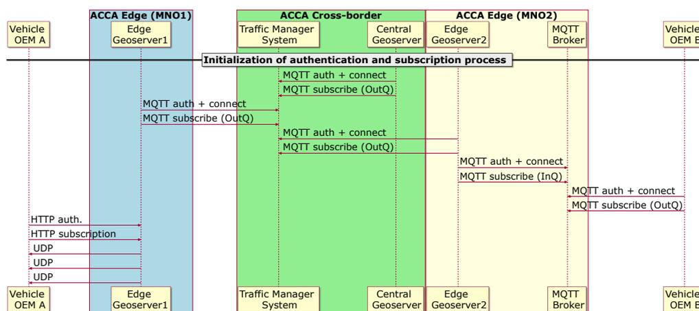
**Figure 2.** Authentication and subscription process for the connectivity establishment between vehicle on-board unit (OBUs) and the backend services on the edge, and between backend services.
