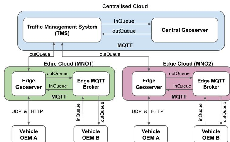
**Figure 1.** Anticipated cooperative collision avoidance (ACCA) service architecture with two connected vehicle original equipment manufacturers (OEMs). Vehicle OEM A communicates over the UDP/IP and HTTP protocols, and vehicle OEM B communicates over the TCP/IP with MQTT protocol.
