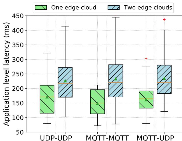
**Figure 8.** Application-level latency between OBUs measured for three different combinations of V2X communication protocols between the sender and the receiver OBUs. One edge cloud represents that both OBUs connected to the same edge cloud, whereas two edge clouds represent that each OBU is connected to a different edge cloud.
