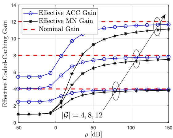
Fig. 5: Effective gain versus  $\rho$  for  $B = 6$ . Right-side plot focuses on realistic SNR values.
