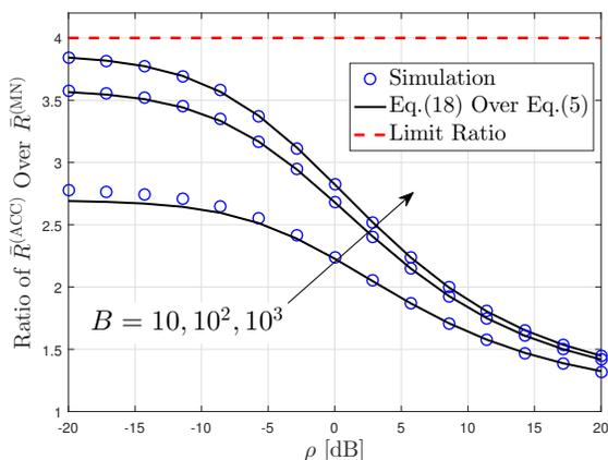
Fig. 11:  $\bar{R}^{(\text{ACC})}/\bar{R}^{(\text{MN})}$  versus  $\rho$  for  $|\mathcal{G}| = 4$ .
