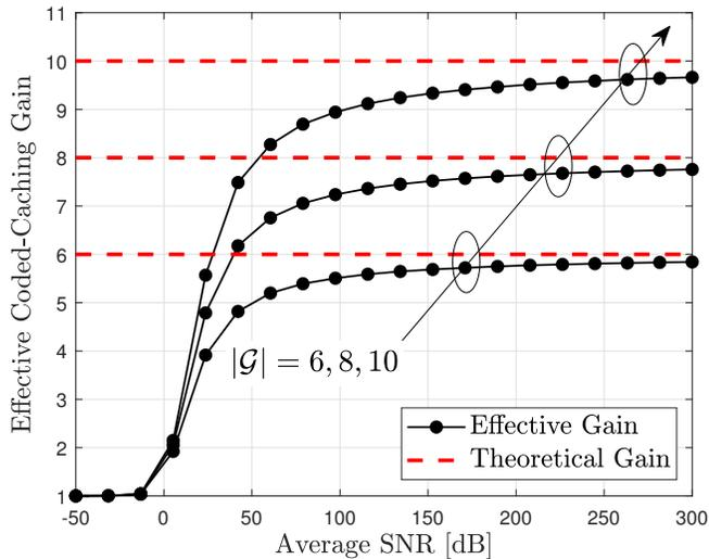
Fig. 1: Ratio between the average rates of the MN scheme and TDM (i.e., the *effective coded-caching gain*) over quasi-static Rayleigh fading channel for different values of  $|\mathcal{G}| = \Lambda\gamma + 1$ .
