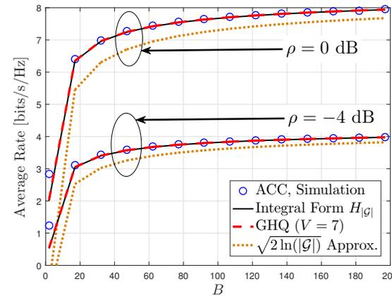
Fig. 9:  $\bar{R}^{(\text{ACC})}$  versus  $B$  for  $|\mathcal{G}| = 10$ .
