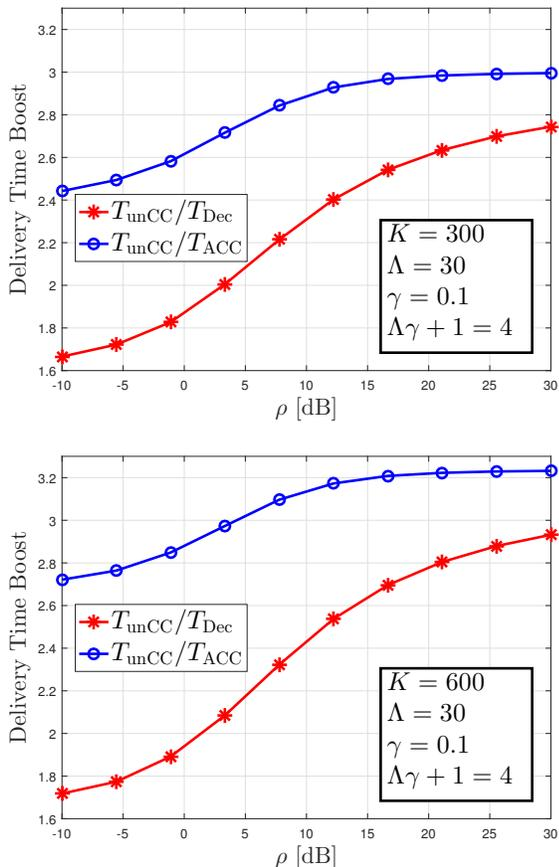
Fig. 12: Comparison of Delivery Time versus  $\rho$  for  $m = 2$  in the decentralized-placement scenario.
