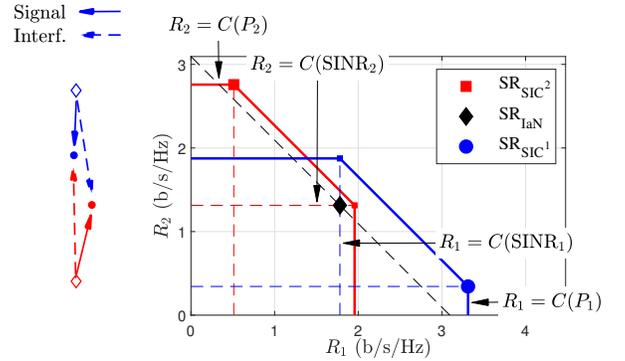
Fig. 1. MAC capacity regions formed by 2 Tx-Rx pairs. Both regions have points above the  $\text{SR}_{\text{IaN}}$  black dashed line (both SIC gain conditions are met).
