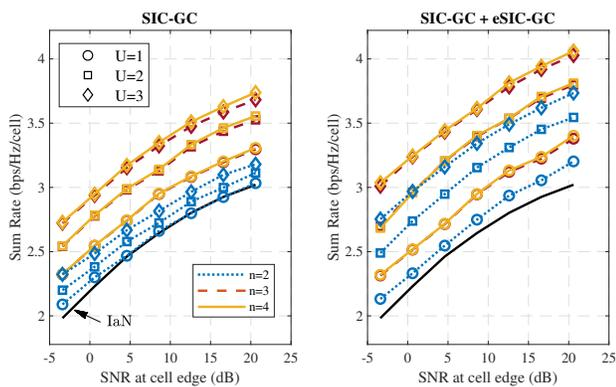
Fig. 5. Per cell sum-rate: IaN vs. Coop-SIC  $n = 2, 3, 4$  and users per cell  $U = 1, 2, 3$ .
