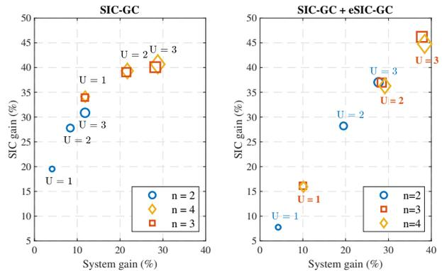
Fig. 6. SIC gain vs. System gain for Coop-SIC orders  $n = 2, 3, 4$  and users per cell  $U = 1, 2, 3$  with SNR = 5 dB at the cell-edge.
