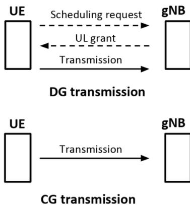
FIGURE 1. UL DG and CG transmission.
