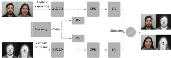
Fig. 1. The proposed SPH framework.
