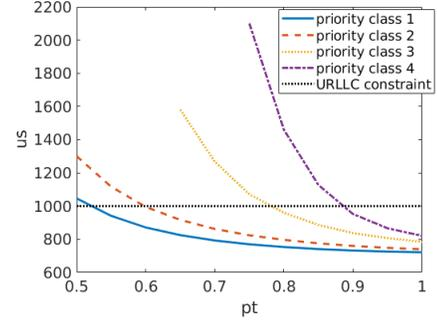
Fig. 6. Total transmission time in UL transmission with 4 repetitions in SCS of 30kHz.
