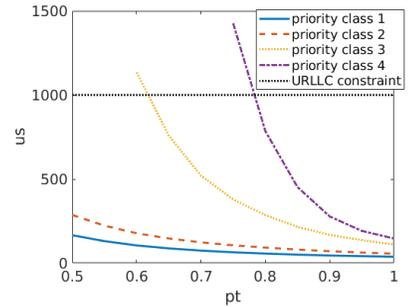
Fig. 2. Type 1 channel access procedures average time in DL transmission.
