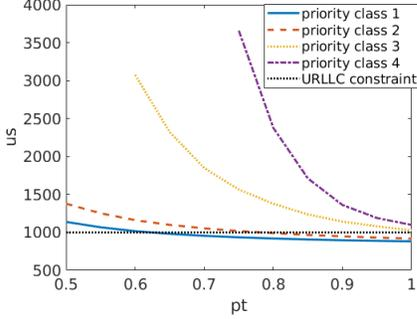
Fig. 4. Total transmission time in DL transmission with an initial transmission and a retransmission in SCS of 30kHz.
