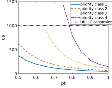
Fig. 3. Type 1 channel access procedures average time in UL transmission.
