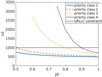
Fig. 5. Total transmission time in DL transmission with an initial transmission and a retransmission in SCS of 60kHz.
