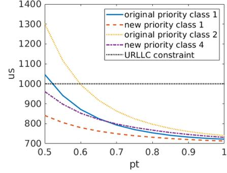
Fig. 8. Comparison of total transmission time between original priority class and new priority class in UL transmission with 4 repetitions in SCS of 60kHz.
