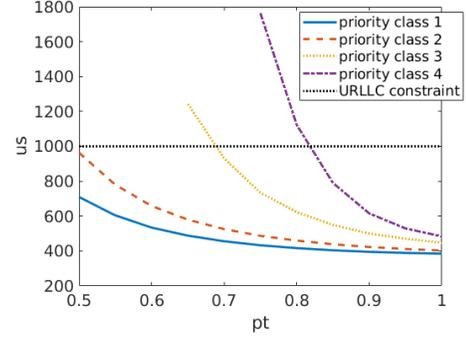
Fig. 7. Total transmission time in UL transmission with 4 repetitions in SCS of 60kHz.
