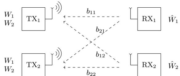
Fig. 1. Cooperative MIMO channel with asymmetric feedback.
