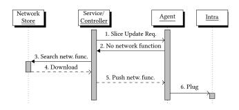
Figure 4: Sequence diagram for CP extension functionality.
