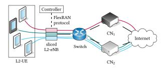
Figure 2: Demo setup using an emulated LTE network (L2-UE, L2-eNB) and two core networks.
