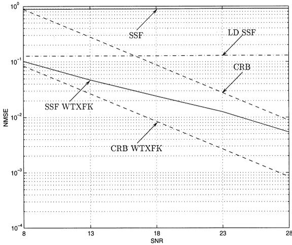
Fig. 4. Performance of SSF, LD SSF and SSF WTXFK.
