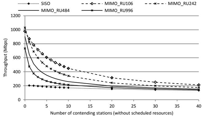
Figure 16. Throughput of UL MU-MIMO with 4 spatial streams as a function of the number of contending stations
