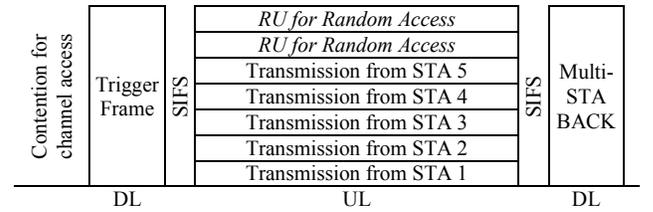
**Figure 1. UL OFDMA transmission with Multi-STA BACK**
