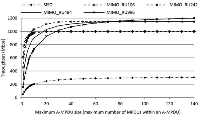
Figure 15. Throughput of UL MU-MIMO with 4 spatial streams as a function of the maximum A-MPDU size
