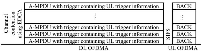
Figure 2. DL OFDMA transmission with UL OFDMA acknowledgement
