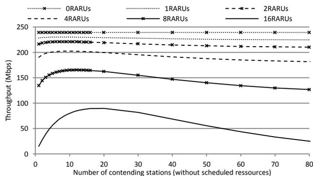
**Figure 7. Throughput of pure UL OFDMA as a function of the number of contending stations**
