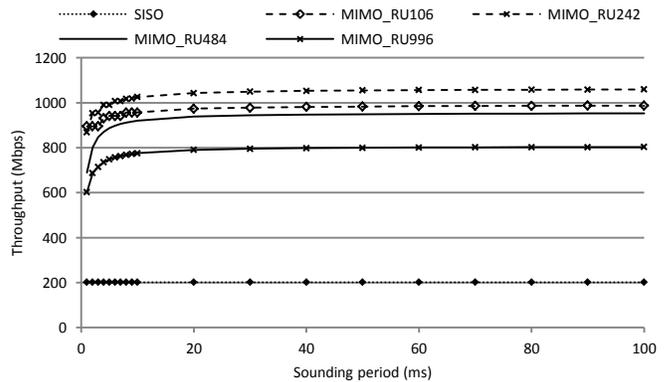
Figure 17. Throughput of DL MU-MIMO with 4 spatial streams as a function of the sounding period
