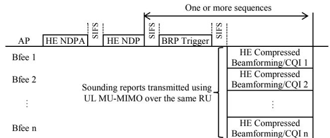
Figure 3. Channel sounding protocol for DL MU-MIMO in 802.11ax
