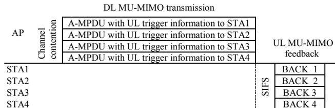
Figure 5. DL MU-MIMO transmission over one RU with UL MU-MIMO feedback
