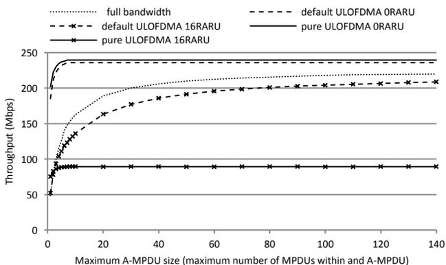
Figure 12. Throughput comparison for different queue sizes
