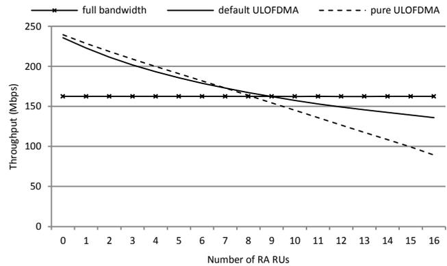
Figure 9. Throughput comparison for different numbers of RA RUs
