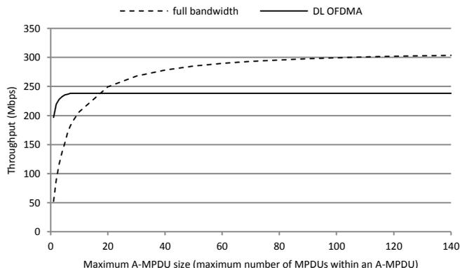
Figure 13. Throughput evaluation of DL OFDMA
