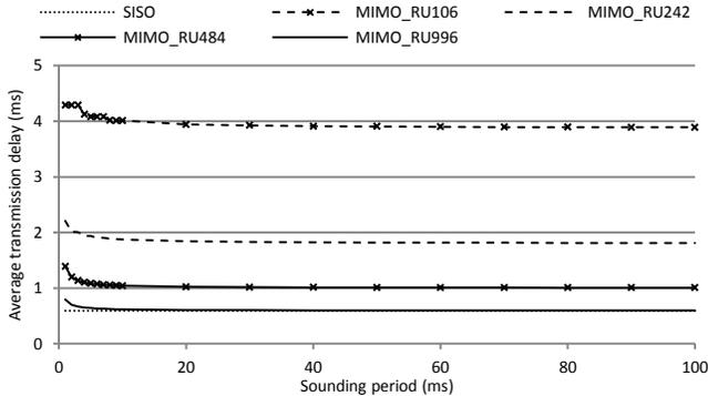
Figure 18. Average transmission delays (in ms) of DL MU-MIMO with 4 spatial streams as a function of the sounding period
