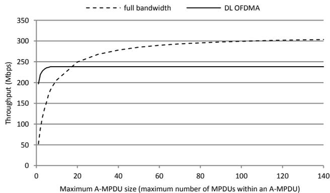
Figure 13. Throughput evaluation of DL OFDMA
