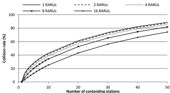
**Figure 6. Collision rate in pure UL OFDMA as a function of the number of contending stations**
