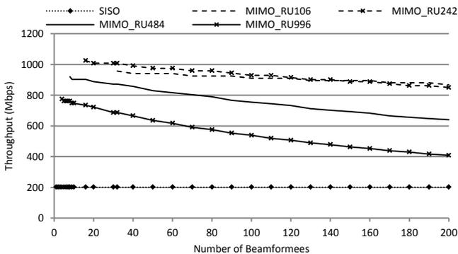
Figure 19. Throughput of DL MU-MIMO with 4 spatial streams and 10ms sounding period as a function of the number of beamformers
