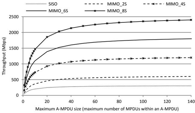
Figure 14. Throughput of UL MU-MIMO using full bandwidth transmissions as a function of the maximum A-MPDU size
