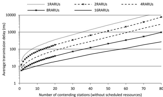
Figure 8. Average transmission delays (in ms) of pure UL OFDMA as a function of the number of contending stations
