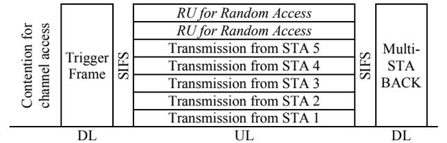
**Figure 1. UL OFDMA transmission with Multi-STA BACK**
