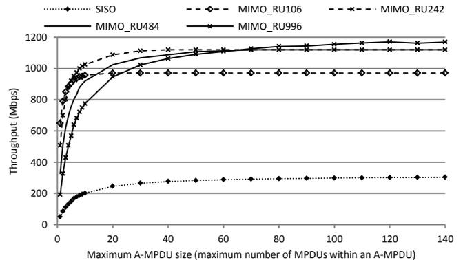
Figure 20. Throughput of DL MU-MIMO with 4 spatial streams and 10ms sounding period for different queue sizes
