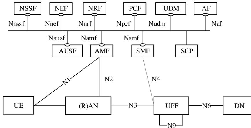
Figure 5: 5G Standalone System Architecture and Interfaces [22].
