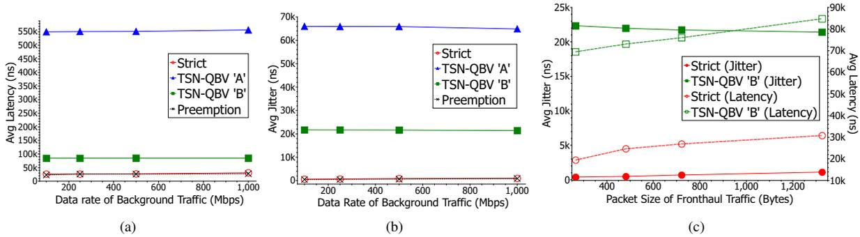
Fig. 5: Evaluation results for fronthaul traffic over (a), (b) varying background traffic and (c) fronthaul packet sizes.
