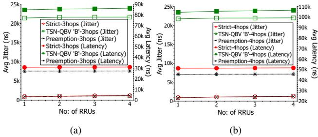
Fig. 6: Jitter and latency for different number of RRUs and hops. Fig.6(a) depicts for 3 hops and Fig.6(b) for 4 hops.
