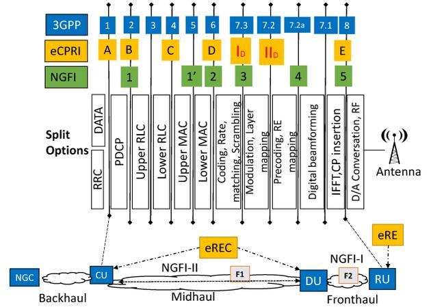
Fig. 1: Functional splits by 3GPP, eCPRI & NGFI (downlink).
